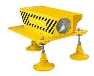
The unit produces a series of coloured signals based on the approach angle of the Helicopter. It will be Flashing Green or Red or Solid Green and Red depending on the angle.
