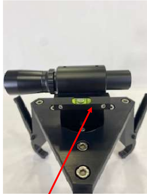
Spirit bubble shows the fitting to be level in this orientation.
