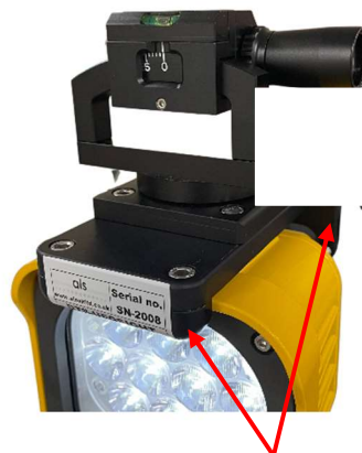
(Fig 3) Position the sighting device carefully over the top of the fitting
