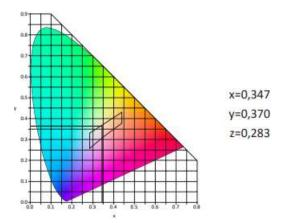
The measured trichromatic coordinates correspond to colour range requirements in: ICAO Annex 14 - Aerodromes Vol.1, fig. A1-1-1b. Colours for aeronautical ground lights (solid state lighting)
