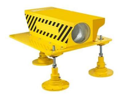
The HAPI unit produces a series of coloured signals based on the approach angle of the Helicopter. It will be Flashing Green or Red or Solid Green and Red depending on the angle.
