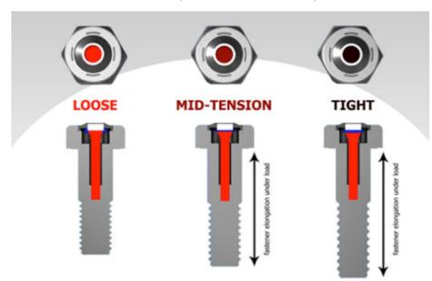
SmartBolts directly correlate tension with colour. Accuracy and reliably is ensured because the colour change of the Visual Indication System is proportional to bolt stretch — the only true measure of how tight your joint is (torque readings alone can be misleading since torque only measures how difficult it is to turn the bolt head).
