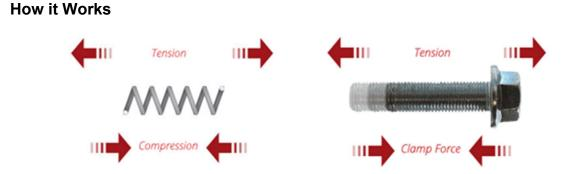
The bolts work very similar to springs. When you stretch a spring, it pulls back – trying to return to its original size. The stretching force is called tension. The force that pulls back is called compression.
