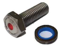
Airfield Lighting Systems (ALS) has launched a Visual Indication System that turns the top head of a bolt from red to black as you tighten it. SmartBolts give you peace of mind because you know your bolts are at the correct tension which is vital for Airfield safety. They can be easily retrofitted to existing runway lighting and do not need to be replaced with every inspection, saving you money and time.
