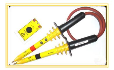
The ALS HV Probe and proving unit have been designed to provide a safe and easy way of proving circuits dead. They prove from 55VAC to 5000VAC. Each unit undergoes rigorous testing before sale, and is serialised for traceability.
